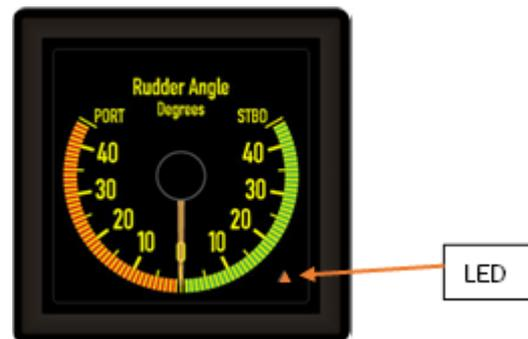
If no new value was stored (switch still closed), wait until >20 seconds. Then the calibration sequence will be terminated without storing a new setting and the indicator pointer will move back to the scale position given by the present rudder transmitter value (normal mode).
