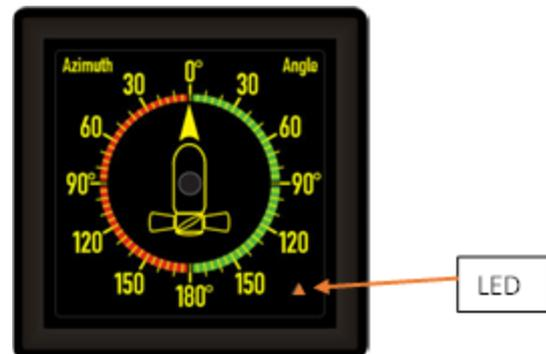
If no new value was stored (switch still closed), wait until >20 seconds. Then the calibration sequence will be terminated without storing a new setting and the indicator pointer will move back to the scale position given by the present azimuth transmitter value (normal mode).
