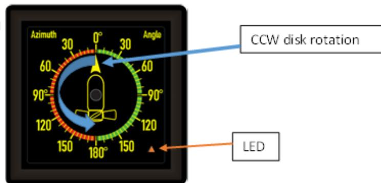
If no new value was stored (switch still closed), wait until >20 seconds. Then the calibration sequence will be terminated without storing a new setting and the indicator pointer will move back to the scale position given by the present azimuth transmitter value (normal mode).
