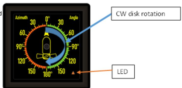
If no new value was stored (switch still closed), wait until >20 seconds. Then the calibration sequence will be terminated without storing a new setting and the indicator pointer will move back to the scale position given by the present azimuth transmitter value (normal mode).
