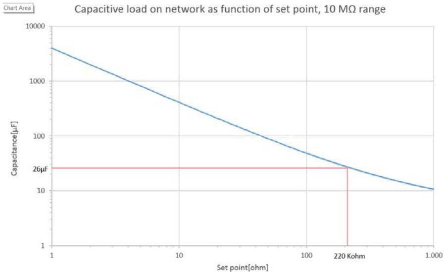
The shown 220 kΩ set point will accept capacitance up to 26 µF on 10 MΩ range, without false warning.
