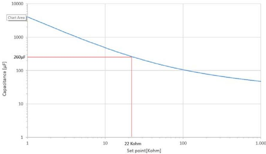
The shown 22 kΩ set point will accept capacitance up to 260 µF on 1 MΩ range, without false warning.
