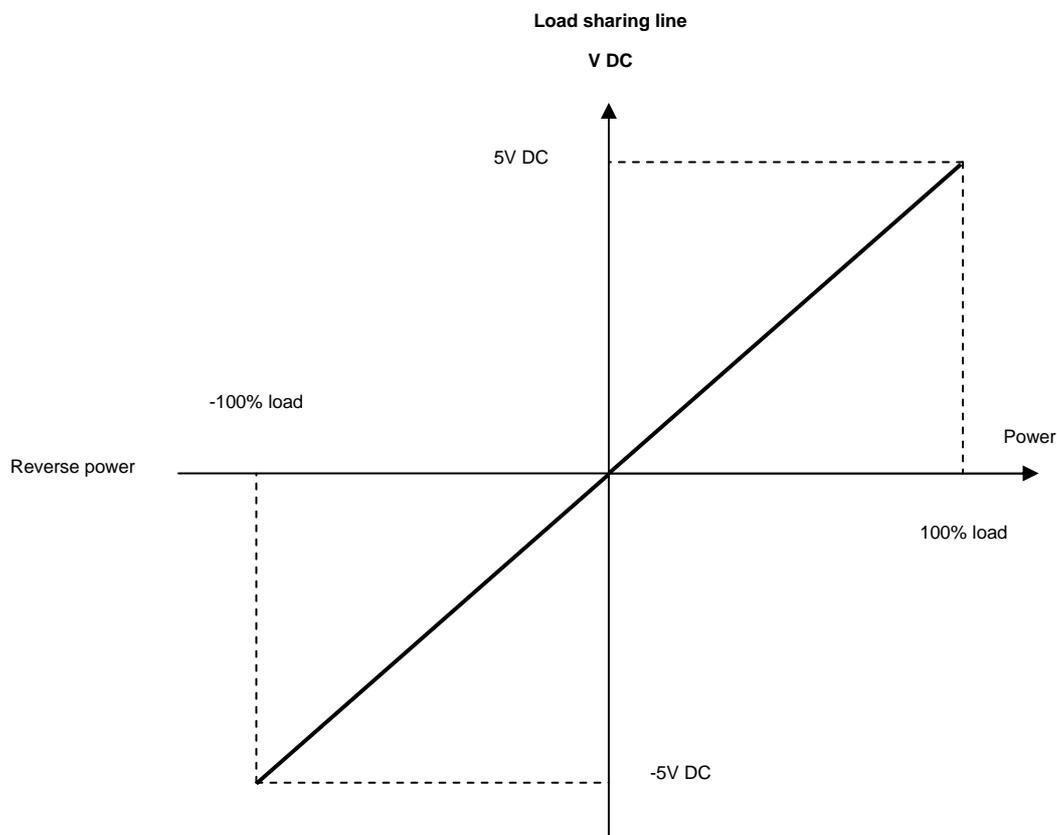
The active load sharing line is illustrated above, and the characteristics of the reactive load sharing line are equivalent to it.
