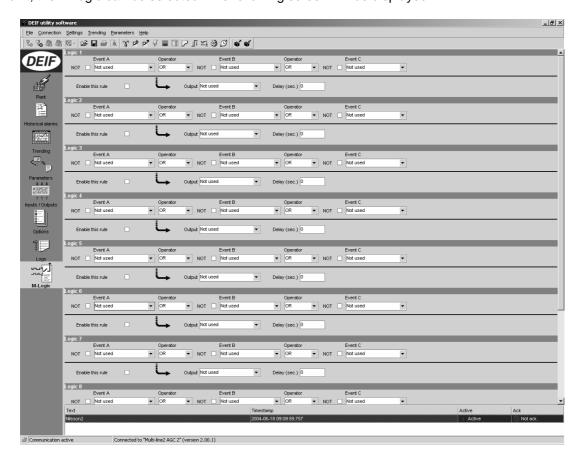
The screen will show the present M-logic configuration. In the example above the M-logic is NOT used.
