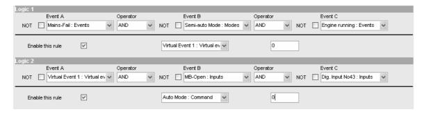
In this example the unit automatically goes to auto mode when these conditions are met:
