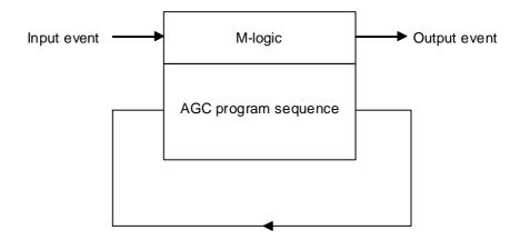
The drawing illustrates the program sequence with the M-logic enabled. M-logic is part of the program sequence.
