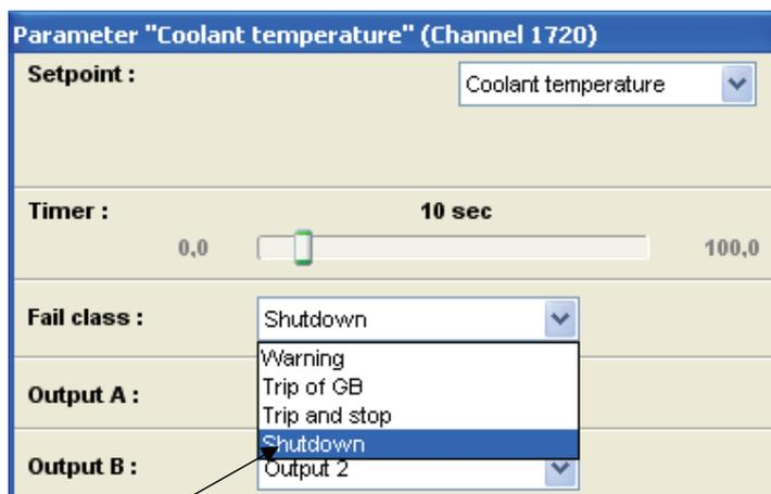
The fail class roll down panel is activated, and the individual functions are ready for selection.
