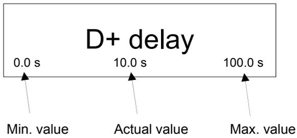
Parameter example: D+ delay setting. Use ▲ or ▼ to scroll through the settings list. If change of settings is necessary, press ↵ and enter the password. Then use ▲ or ▼ to change values. Press ↵ to save setting. Use ESC to leave settings.
