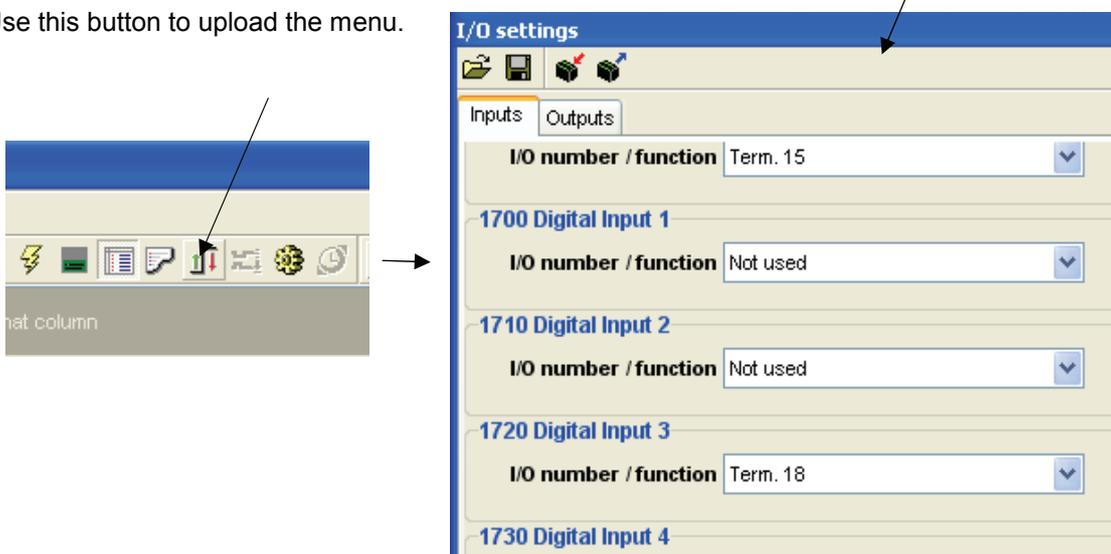
The individual I/O number and the function are now selected. In the example below 'Digital input 3' is chosen, and a terminal number must be assigned to the input. If the input is used as alarm input, then the name can be changed to the relevant name selected from the predefined list below:
