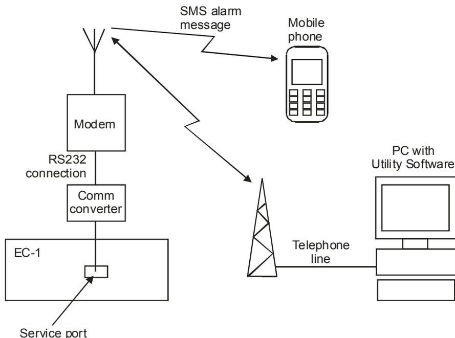
The connection is based on an RS232 connection to a GSM modem via the service port on the EC-1/EC-1M. Since the connection on the EC-1/EC-1M is a TTL communication, the interface box PI-1 (option J5) is needed to convert the signals to RS232. The PI-1 connects via a cable with SUB-D 9-pin female connector on the modem side.
