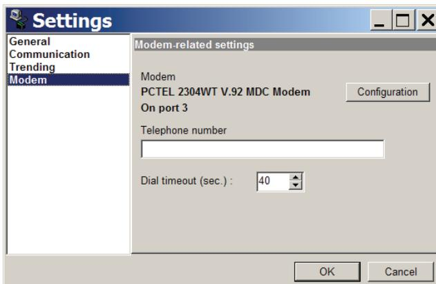
Select modem and key in the telephone number of your GSM modem connected to the unit.
