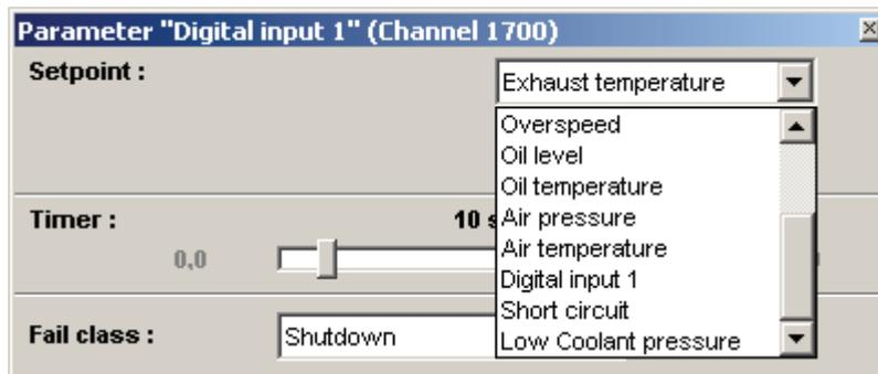
Complete the input settings and select the appropriate fail class and outputs. The outputs A and B can be used to activate one or two of the configurable relay outputs. If the relay function is set as a limit relay, no warning pop-up will be shown in the display. The relay 0 is a virtual relay, so both output A and B must be set to limit relays if no warning in the display is wanted.
