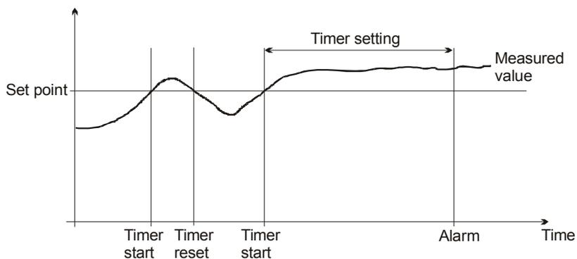
When the timer runs out and the alarm is present, the output is activated.
