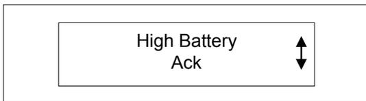
**Active alarm list.** The alarm list automatically pops up, when an alarm appears. When the arrow is present, more alarms are active. Press **▲** to scroll through the list. Exit the list by pressing ESC.
