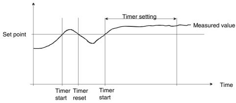
When the timer runs out, the output is activated.
