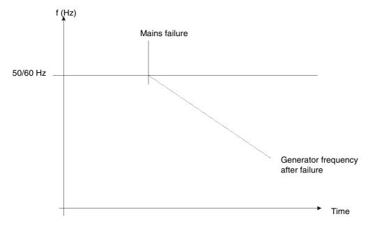
So, a dramatic drop of frequency over time is a mains failure.
