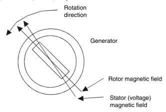
If a mains failure occurs, the time lagging of the stator magnetic field (and the output voltage) will change (jump) and that is called the vector jump.
