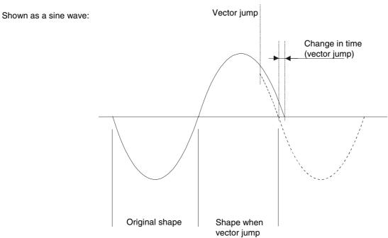
So, by comparing the half-sine curve time duration with the previous ones, a sudden change in time can be detected. This is the vector jump.
