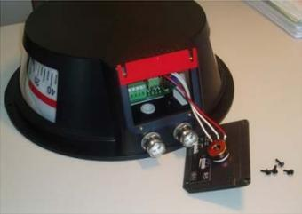
Remove the rear plate (4 screws).
