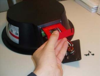
Gently draw the transport lock out with a hand. When inserting the transport lock again, gently insert it between the scale guide (white plastic part inside) and the housing (black part).
