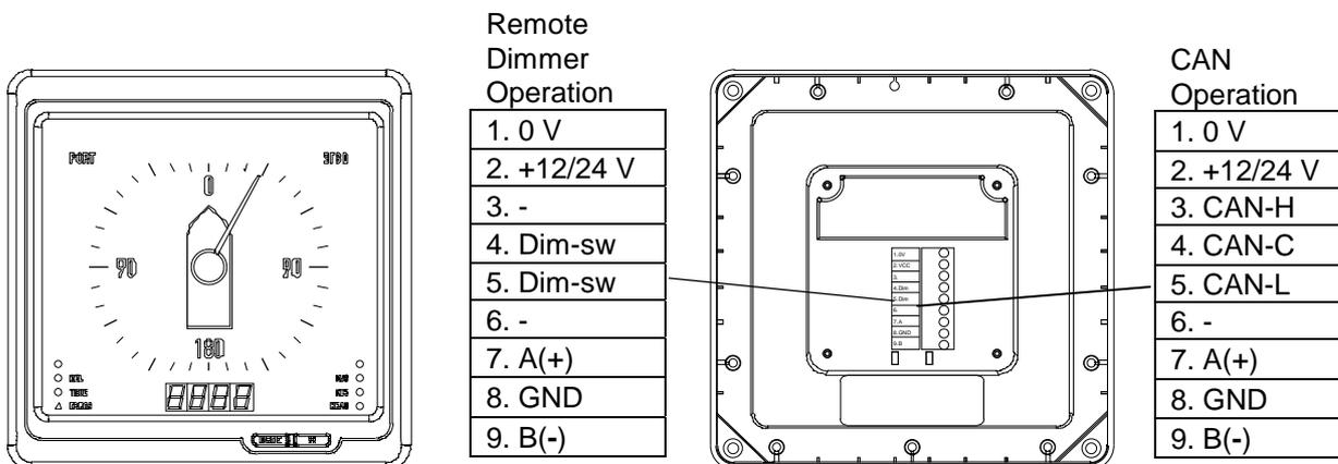
**i** Terminal no. 4 and no. 5 is either used as “remote dimmer input” or as part of the CANbus. Remote dimmer and CANbus cannot be used at the same time!
