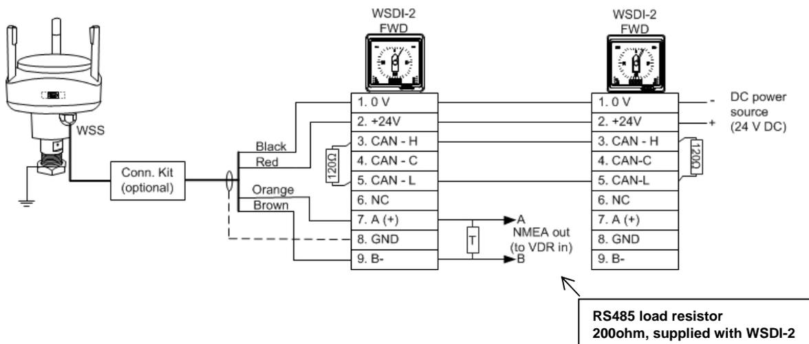
CANbus must be terminated in both ends.
