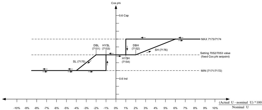
**i** The settings of MA and MI can be reversed, meaning that the reactive power will move in the inductive direction with increasing voltage.
