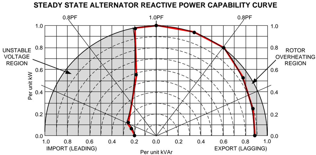
The settings of points 1-6, leading and lagging, should represent the generator manufacturer's recommended settings for var import (-Q)/export (+Q). Notice that the above curve is just an example, the actual values must be obtained from the generator manufacturer.
