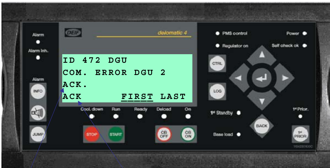
The ACK status line in the display The ACK must have an active underline when acknowledging
