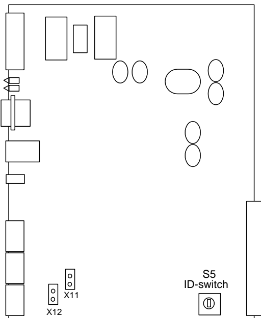
Address switch/jumpers on the PCM module
