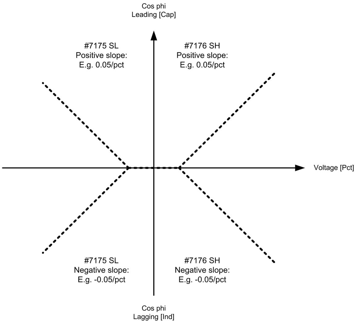
When the requirement of the voltage support is known, it can be decided whether the slope is positive or negative. This is best illustrated with an example:
