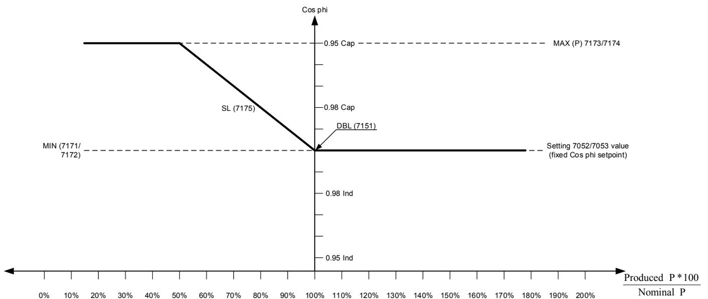
The system measures and reacts based on the generator power measurement. The function will make a dynamic power-dependent cos phi that is used to support the mains voltage/compensate the voltage impact of the power produced. The ramp has a
