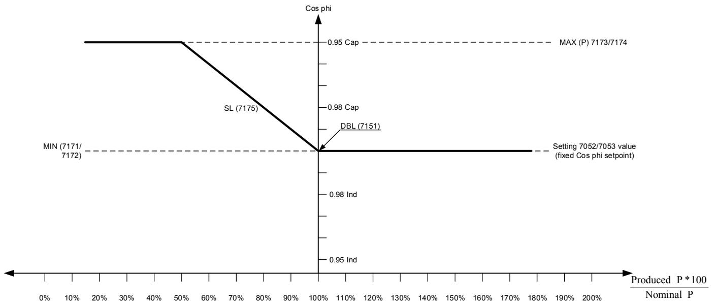
The system measures and reacts based on the generator power measurement. The function will make a dynamic power-dependent cos phi that is used to support the mains voltage/compensate the voltage impact of the power produced. The ramp has a configurable deadband (DBH) that can be used with reference to the nominal power of the generator to deactivate the ramp functionality.
