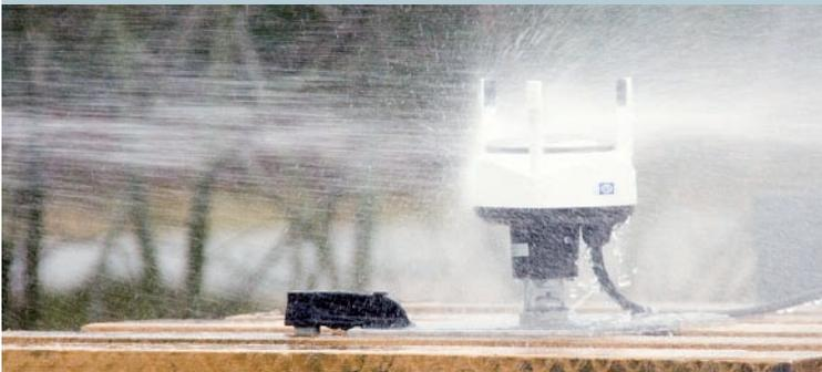
Water protection test, IP66
